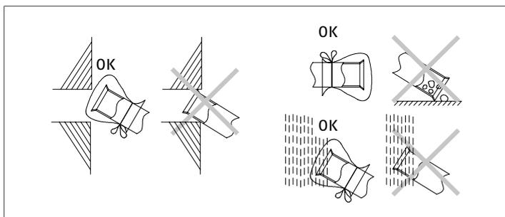
**⚠** Plug the pipe ends in order to prevent water or debris from flowing in.
