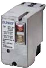
To test the valve seals on the gas train, a special "seal control kit" is available. The valve seal control device is compulsory (EN 676) on gas trains to burners with a maximum output over 1200 kW. The sealing control is type VPS 504.
