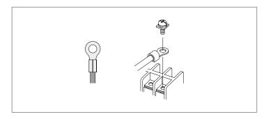
It is compulsory to use ring crimp terminals to connect to the terminal board.
