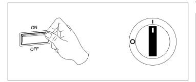
— position the system's main switch in the "ON" position.
