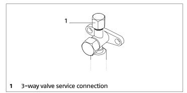
charge the circuit with nitrogen through the service connection on the 3-way shut-off valve
