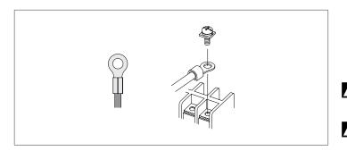
🛕 It is compulsory to use ring crimp terminals to connect to the terminal board.
