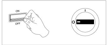
— position the system's main switch in the "OFF" position.
