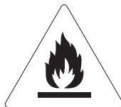
Caution: Risk of fire/ flammable materials
