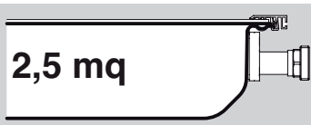
Collettore 2,5 mq VERTICALE con VASCA con 2 attacchi G 1" 2.5 m 2 VERTICALLY MOUNTED COLLECTOR with TRAY and 2 x G 1" fittings
