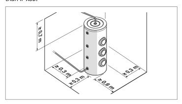
NOTE: the above-indicated dimensions are recommended for a correct maintenance and access to the device.
