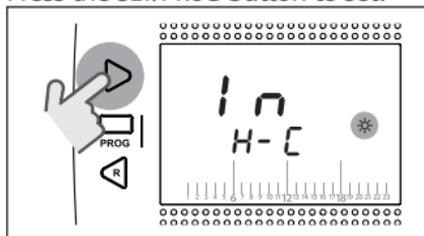
Press the UP ^ or DOWN v button to select the desired mode.
