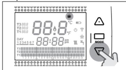
**!** The room setpoint temperature set cannot be higher than or equal to T3 (comfort) or less than or equal to T1 (anti-freeze).
