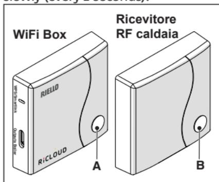
Press the prismatic dome clear LED button (B) on the boiler RF receiver and hold for 5 seconds until the green and red LEDs flash frequently (every 0.5 seconds) at the same time.
