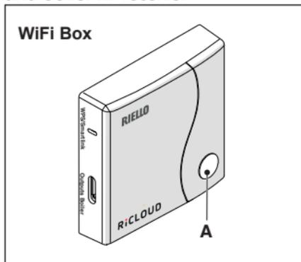
In case of a boiler alarm (available with OTBus connection between the WiFi Box and the boiler or the RF receiver and the boiler or **RiCLOUD** and the boiler, if provided for by the OT-Bus protocol), the alarm can be reset by pressing the prismatic dome clear LED button (A) (for alarm A99, reset from the boiler).
