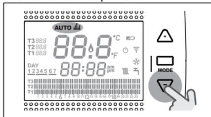
Press the SET/PROG button to save and return to the HOME screen, press ESC/MODE to save and return to the HOME screen, or wait 5 seconds to automatically save the value and return to the HOME screen.
