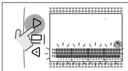
Press the SET/PROG button to set. Press the FORWARD > or BACK < button to select the day or period of the week to be changed.
