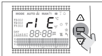
Once the system pressure has been restored, **RiCLOUD** automatically returns to the normal HOME screen display.
