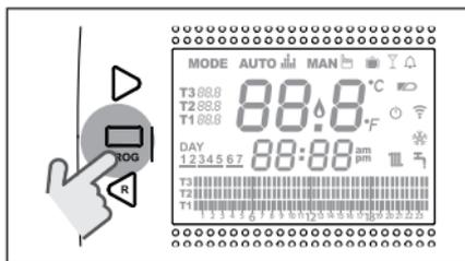
Press the FORWARD > or BACK < button to select the field HEATING/COOLING TIME PROGRAM.
