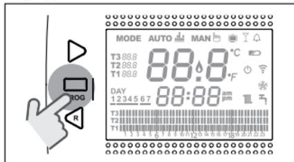
Press the FORWARD > or BACK < button to select the field HEATING/COOLING.
