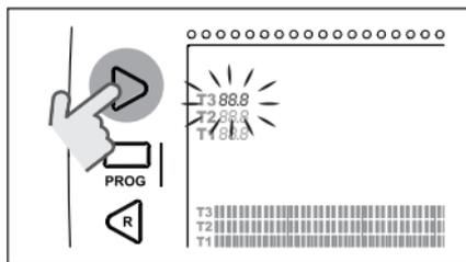
Press the UP ^ or DOWN v button to modify the selected room setpoint temperature.
