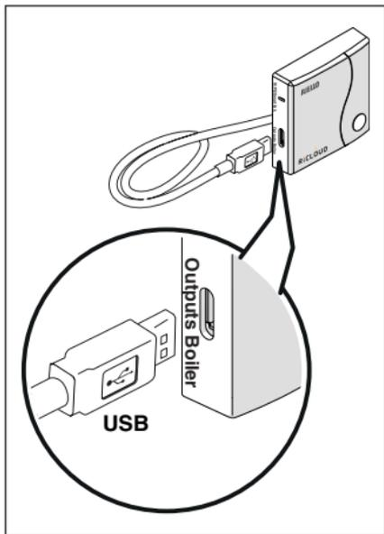
Power the WiFi Box via the relevant cable and power adapter provided.
