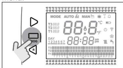
Press the FORWARD > or BACK < button to select the field DHW TIME PROGRAM.
