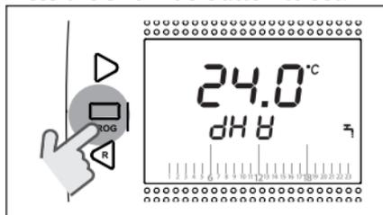
Press the UP  $\wedge$  or DOWN  $\vee$  button to modify the domestic hot water setpoint temperature.
