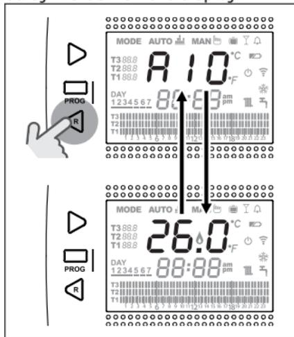
In case of a boiler alarm (available with OTBus connection between the WiFi Box and the boiler, if provided for by the OTBus protocol), the alarm can be reset by pressing the BACK/RESET button < (for alarm A99, reset from the boiler).
