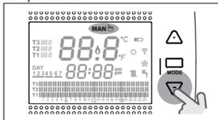
**!** The room setpoint temperature set cannot be less than or equal to the T2 temperature (economy).
