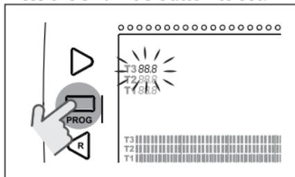
Press the FORWARD > or BACK < button to select the temperature to be changed.
