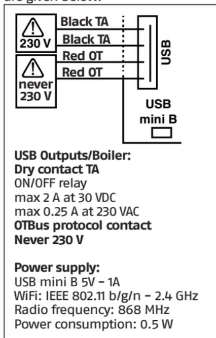
Two USB cables are also supplied, one to provide power via the USB power adapter and the other to connect the WiFi Box to the boiler. The cable to connect it to the electrical power supply is a USB mini.
