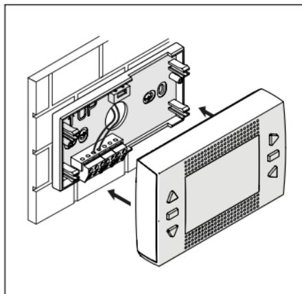
Re-attach the **RiCLOUD** thermostat to the wall plate by aligning and then pressing firmly around the outer edges.
