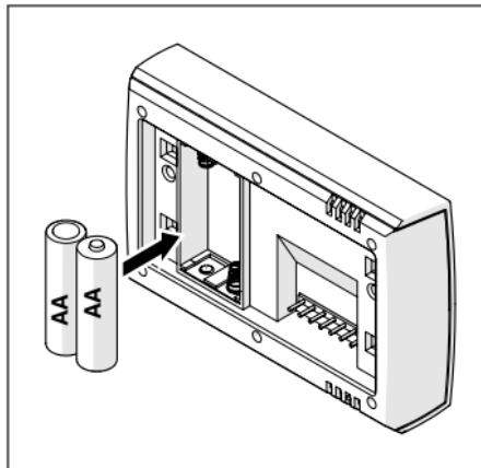
Insert two 'AA' type batteries (supplied), into the battery compartment.
