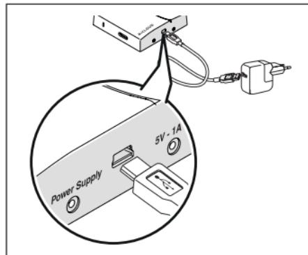
*Using the mini USB cable and power adaptor (supplied); connect the WiFi box to an adjacent electrical socket .*
