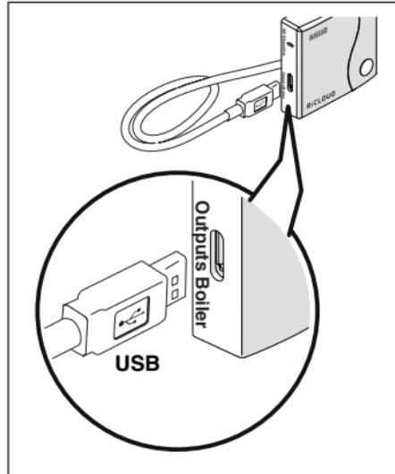
*In case of wireless installation, insert the other end of the USB cable into the OUTPUTS/BOILER socket of the WiFi Box.*
